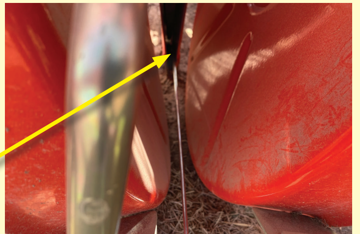
Clean-out rod to clean out soil/debris from throat and shoes.
