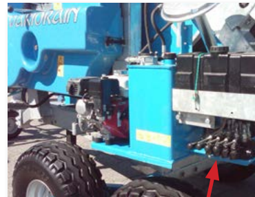
Optional hydraulic Honda engine drive with 4 levers (reel, stabilizer legs, tongue jack and turntable)
