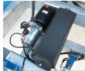
Optional electric motor with solar panel to run machine hydraulics (no tractor needed)
