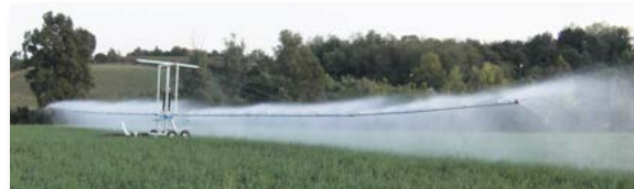
OCMIS low-pressure booms range from 60'-164' irrigated width-- 85% uniformity. (other brand available up to 250')
