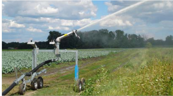
OCMIS offers the offset guncart option to avoid having the hose drag through your crops. 4-wheel cart is standard on 3" machines and above.
