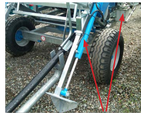
Standard hydraulic hand-crank stabilizer legs/cart-lift (optional for model R2/2 and smaller)
